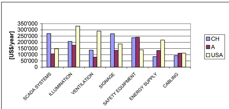
FIGURE 11 – AVERAGE REPLACEMENT COSTS PER ANNUM FOR 3 TYPICAL TUNNELS BASED ON – AVERAGE LIFE CYCLES COLLECTED IN THE SURVEY
