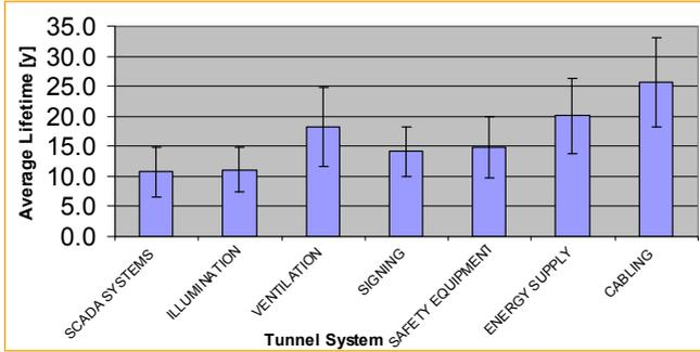
FIGURE 10 - STANDARD DEVIATIONS IN YEARS, MAX/MIN DEVIATIONS
