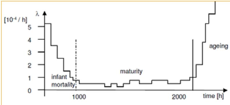
FIGURE 5 - EXPERIMENTAL FAILURE RATE
