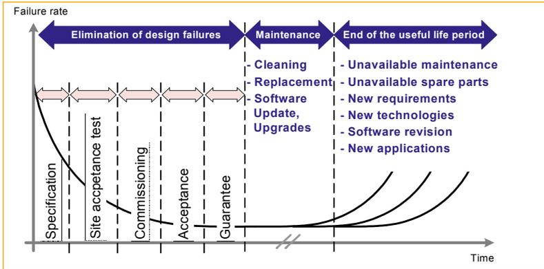
FIGURE 20 - ADAPTED BATHTUB CURVE FOR TECHNICAL EQUIPMENT INCORPORATING SOFTWARE
